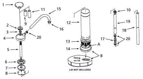
Figure 1 — Replacement Parts Illustration
