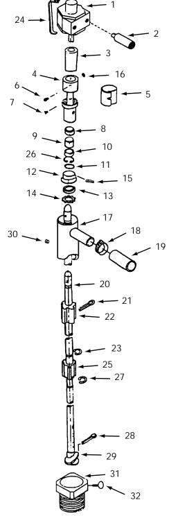
Figure 1 — Replacement Parts Illustration for Model ACT-12NSS
